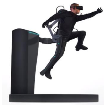
Figure 25 shows a more compact design wherein the user can be rotated in most degrees of freedom as well. Both need a fixed point to rotate the person. It makes the most sense attaching it near the centroid of the user, near the hips.
